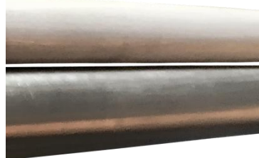
Figure 3 Annealed & Pickled, Polished 320 Grit Tube
