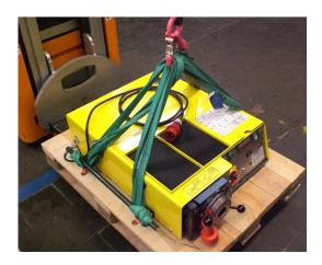
For the transport use only and exclusively suitable transport packaging and slinggear (see illustration). Handles are supposed to be used as fixing points.
