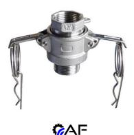
Cam and groove fittings are used to build connection between hoses and pipes. Cam-lock fittings are used in liquid applications or dry bulk applications, but not to be used for air or steam applications. It is available in aluminium material, stainless steel material, and brass material to suit application in various sectors.
